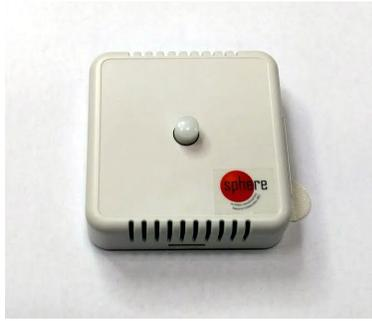
**Figure 5:** SPHERE Environmental Sensor node.
