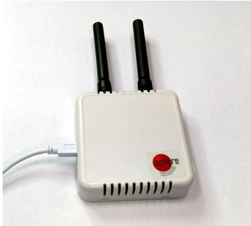
**Figure 7:** SPHERE Forwarding Gateway node.
