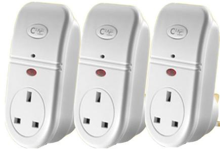
**Figure 8:** Appliance monitor (*CurrentCost*) sensor nodes.
